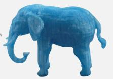
Printed model with support structure removed
